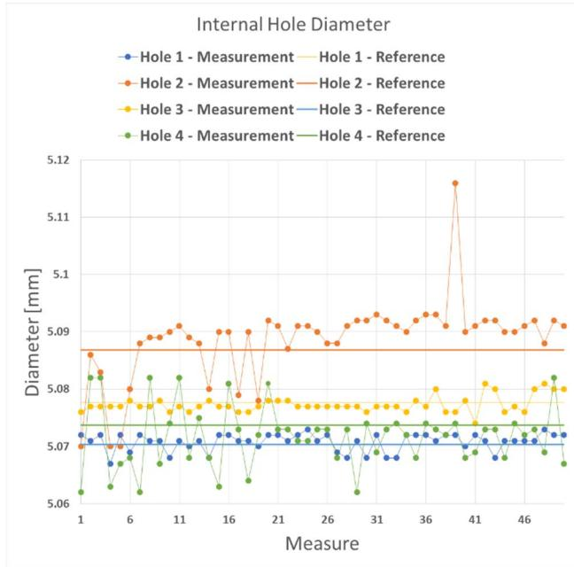
Fig. 15. Internal hole diameter measured with 2D Smart Inspection Tool
