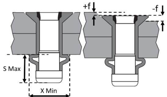
Fig. 4. Fastener Sleeve and Flushness installation limits
