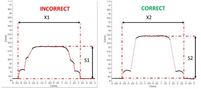
Fig. 13. Example of geometrical feature extraction on a corrected installed and defected fastener sleeve
