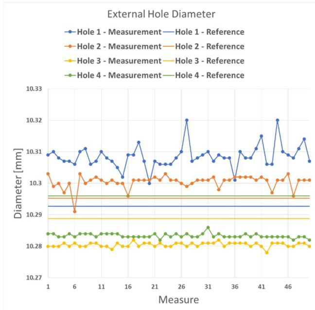
Fig. 16. External countersink hole diameter measured with 2D Smart Inspection Tool
