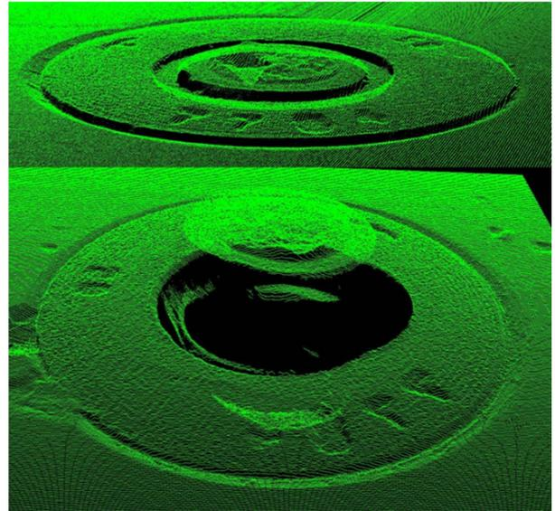
Fig. 12. Correct installed and defected fastener head (point cloud)
