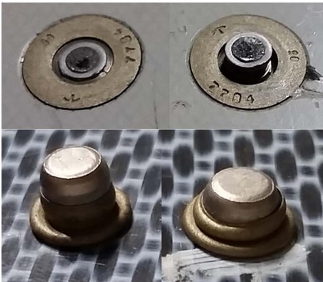
Fig. 10. Correct installed and defected fastener head and sleeve
