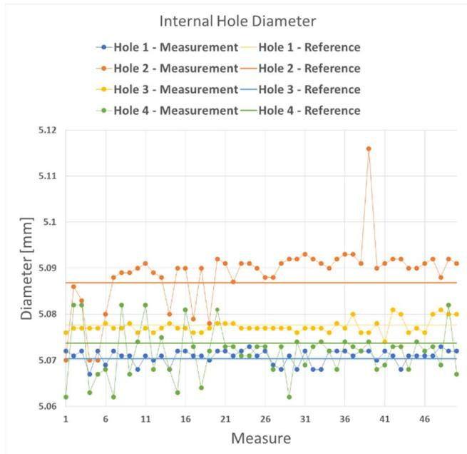
Fig. 15. Internal hole diameter measured with 2D Smart Inspection Tool
