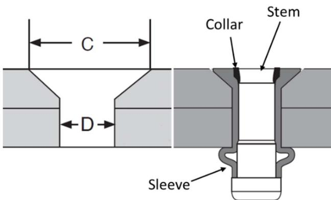
Fig. 1. Holes parameters and fasteners components
