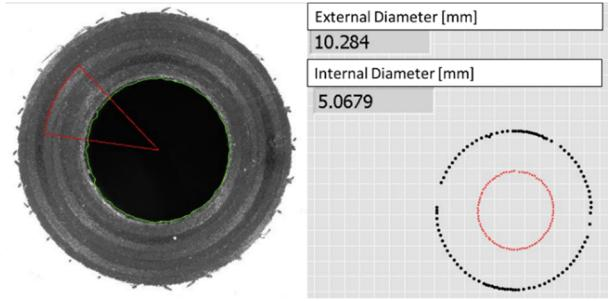
Fig. 6. Image acquired (left); Image elaboration (right)
