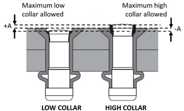
Fig. 3. Fastener Collar installation limits
