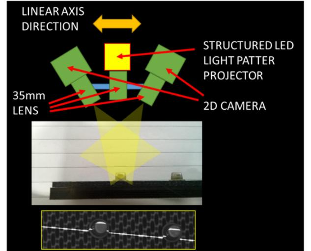
Fig. 7. 3D Smart Inspection Tool
