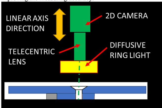
Fig. 5. 2D Smart Inspection Tool
