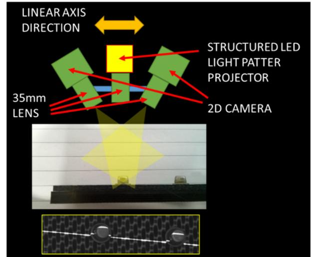
Fig. 7. 3D Smart Inspection Tool
