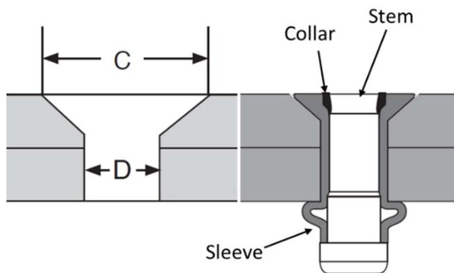
Fig. 1. Holes parameters and fasteners components
