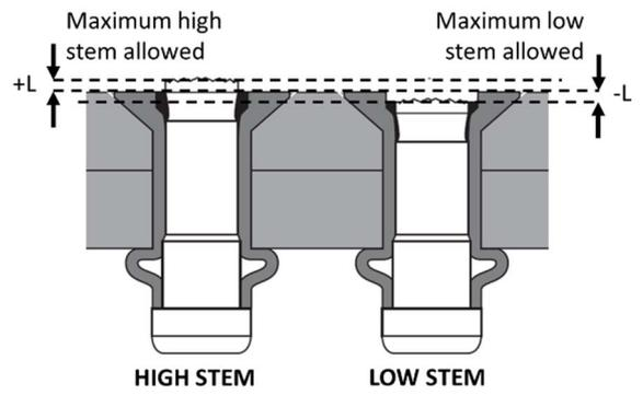
Fig. 2. Fastener Stem installation limits
