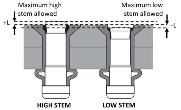
Fig. 2. Fastener Stem installation limits
