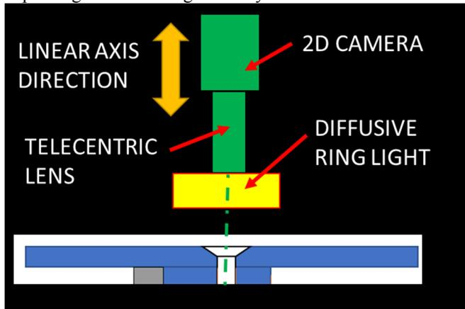
Fig. 5. 2D Smart Inspection Tool
