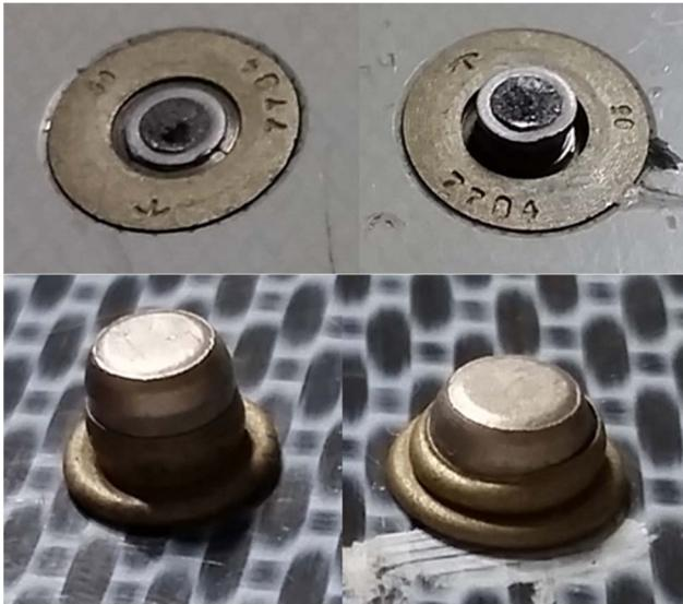
Fig. 10. Correct installed and defected fastener head and sleeve
