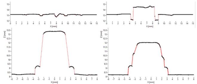
Fig. 11. Correct installed and defected fastener head and sleeve (profile)
