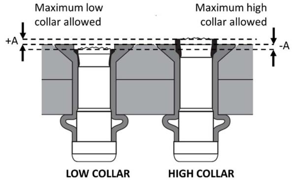
Fig. 3. Fastener Collar installation limits
